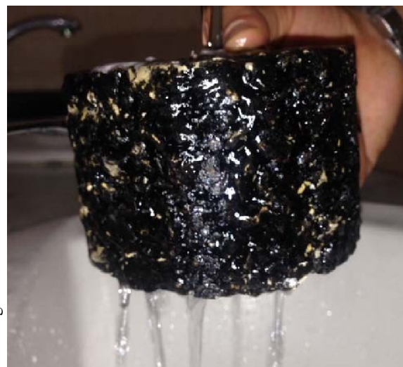
Figure (3): Porous asphalt specimen while permeability test
