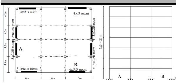
A seven-story building frame system (residential) with shear walls has the dimensions shown in the Figure. The total sustained dead load is 800 kg/m2. This building is located in Gaza Strip and lies on top of a deep clayey deposit( $S_D$ ). Eight shear walls, with the dimensions shown in the figure a lateral force resisting system. Determine the seismic shear loads at the fourth story level acting on shear wall A& B using 1997 UBC.
