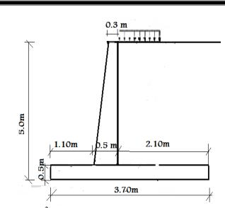
If you know that the allowable net bearing capacity=180 KN/m<sup>2</sup> and the angle of friction and cohesion *of soil under the base of retaining wall are*  $\emptyset = 33^{\circ} \& 9.0$ KN/m<sup>2</sup> respectively, Check the stability for the shown concrete cantilever retaining wall designed to resist earth pressure of soil with  $\emptyset = 28.5^{\circ}$ ,  $\gamma = 16.3$  KN/m<sup>3</sup> and surcharge of 35 KN/m<sup>2</sup>
